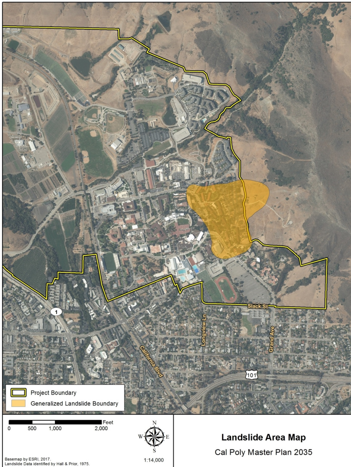
Figure 38. Existing Landslide Boundary
